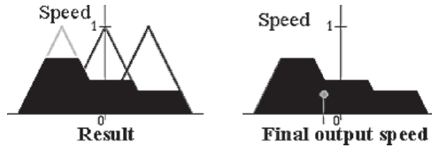
Fig. 1.40. Left: Overlapping single-rule results to yield the overall result. Right: The result of the fuzzy controller so far is a fuzzy set (of speed), so we have to choose one representative value as the final output; there are several heuristic defuzzification methods, one of them is to take the center of gravity of the fuzzy set. This is called Mamdani fuzzy controller .
