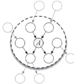
Fig. 1.6. A generic Markov blanket: the set of nodes MB(A) composed of A 's parents, its children, and its children's parents.
