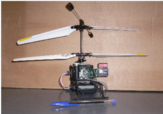
Fig. 1. Helicopter retrofitted with the new electronics, the Gumstix computer and the IMU
