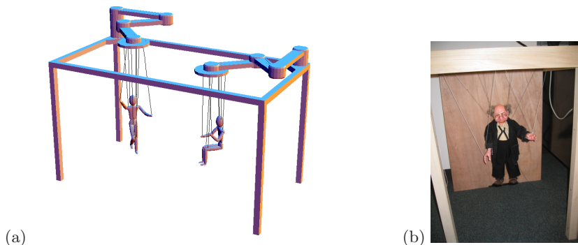
Fig. 1. A Mathematica graphical representation of the mechanical system for autonomous puppetry control (a), together with one of the marionettes used (b)
