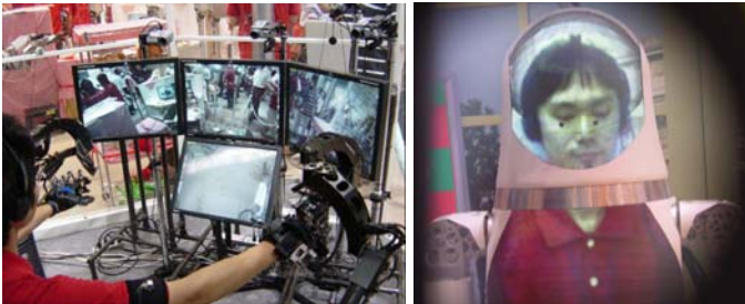
Fig. 9.12. Mutual tele-existence system: master operating cockpit (left), and projection slave (right), (Courtesy of R. Tadakuma and S. Tachi, the University of Tokyo)
