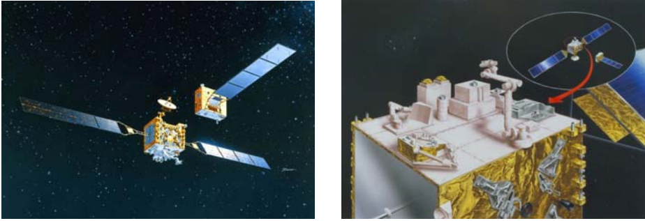
Fig. 19.5. The ETS-VII satellite was designed to verify key technologies on autonomous rendezvous, docking (left) and robotics technologies in space (right). To experiment the rendezvous-and-docking maneuver HIKOBOSHI had opened the docking mechanism holding ORIHIME and started to separate from each other at the low speed of 2cm/sec. After separation HIKOBOSHI and ORIHIME flew in formation for several minutes at a constant distance. On command HIKOBOSHI started approaching ORIHIME along the flight direction (1cm/sec) and captured ORIHIME with the docking mechanism [45]. [Photos by courtesy of JAXA].
