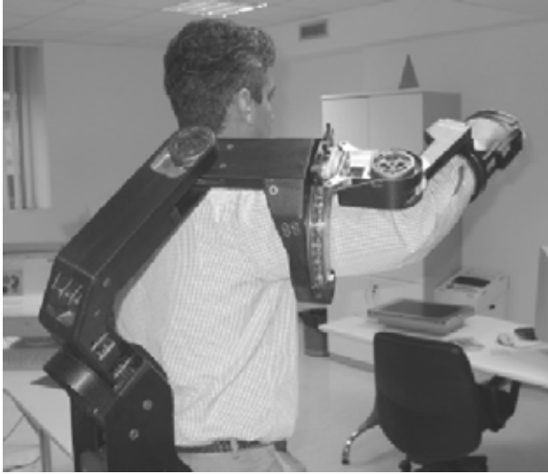
Fig. 4.14. Rear view of the L-Exos in an extended posture, (PERCRO, 2003)
