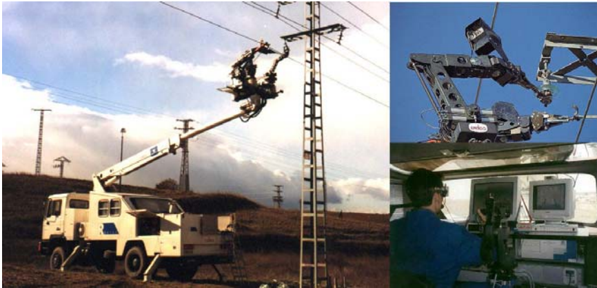
Fig. 27.2. General view of Robtet system (left), robot working site (top-right) and operator working site (bottom-right)
