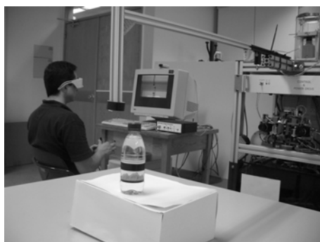
Fig. 5.9. Experiment Setup. Operator is guiding a mobile platform using mono and stereoscopic images.
