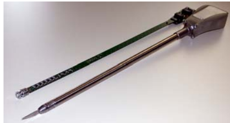
Fig. 21.4. Sensorized scalpel with force/torque sensor at tip and electronics
