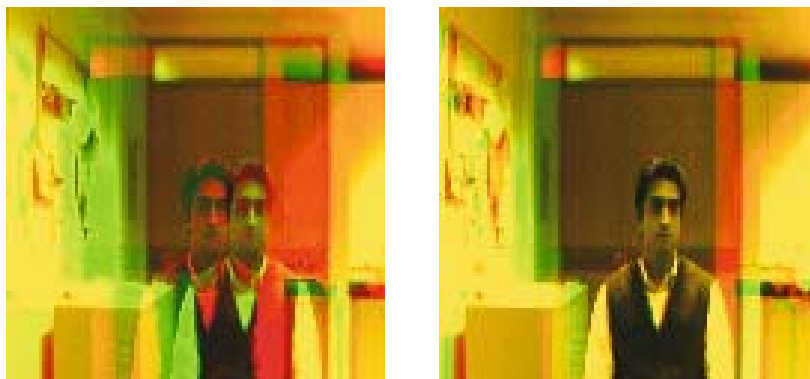
Fig. 5.8. Active vergence experiment. Images from the left and right cameras have been blended for display purposes. The left figure represents the initial state (not verged), where the disparity in the person in front of the setup is noticeable. The right figure shows the system state after convergence, when disparity in the person is cancelled.
