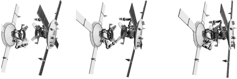
Fig. 19.13. The capturing approach of the floating, non-cooperative target system: (1) Close approach phase, (2) capture of the target by chaser with the aid of manipulator, and (3) pulling along guide elements of Docking Units and fixation with the help of locks of Docking Units
