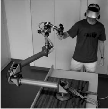
Fig. 2.1. ViSHARD6 prototype (left) and its singularity free translational workspace for an orientation workspace of 360^\circ , 90^\circ , and 360^\circ for the angle of roll, pitch, and yaw, respectively (right)
