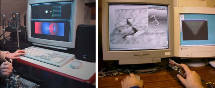
Fig. 9.8. Examples of nano-telemanipulators using AFM. Left image illustrates the ICA-INPG interactive nano-telemanipulator [17]: the AFM (left to the computer screen) is controlled through a gesture/haptic transducer (held by the right hand), computer screen shows visualization of the nano-interaction forces that occur between the cantilever’s tip and the explored surface; forces are amplified and rendered through a haptic transducer; audio substitution of some interaction phenomena is also rendered. Right image illustrates a nano-telemanipulation using one degree of freedom haptic interface for tapping operations; left screen shows the obtained scanned image and right screen AFM cantilever’s tip (courtesy of the University of Tokyo [18]).
