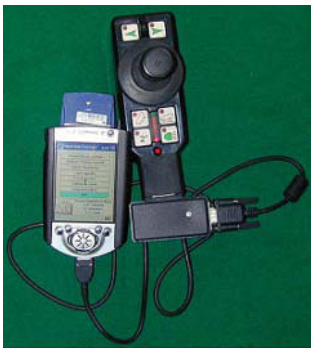
Fig. 24.4. Joystick-activated HMI prototype
