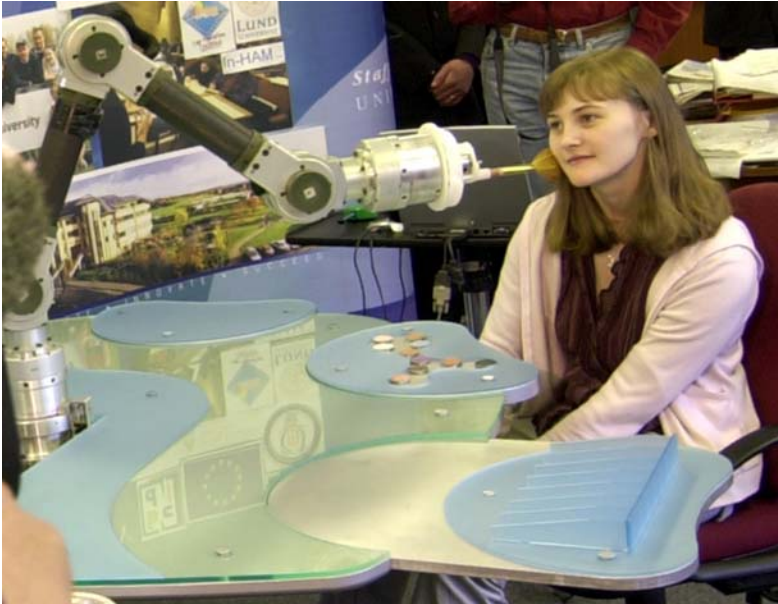
Fig. 24.8. Making-up task assistance by ASIBOT
