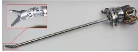
Fig. 21.5. Sensorized pair of forceps, with force/torque sensor and two additional DoF at distal end as well as drive unit at proximal end
