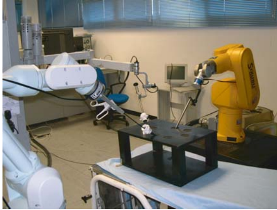
Fig. 23.5. Experimental operating room showing the surgical robots working on a patient simulator. Form left to right: RX-60, ERM, and PA-10.
