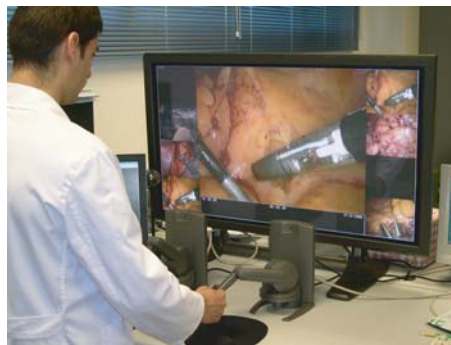
Fig. 23.2. Telesurgery workstation with force feedback master manipulators
