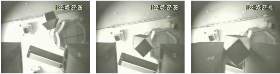
Fig. 19.4. One of the pioneering experiments in ROTEX was the fully automatic grasping of a free-flying object from ground despite a varying round-trip-delay of up to 7 seconds
