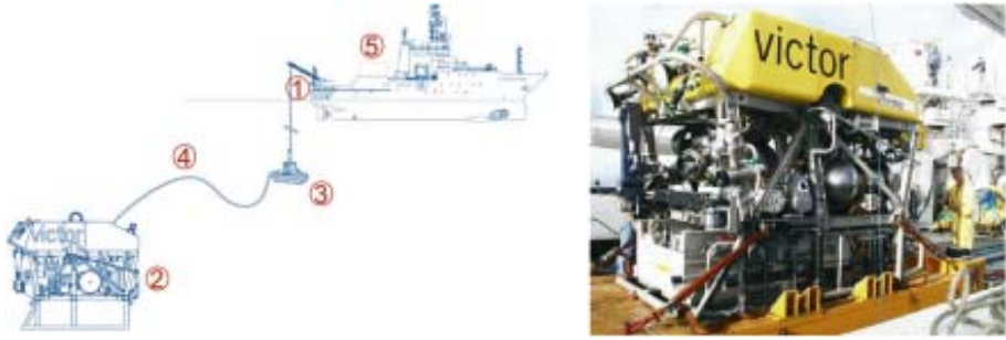
Fig. 20.2. Deep ocean ROV VICTOR 6000 (IFREMER)
