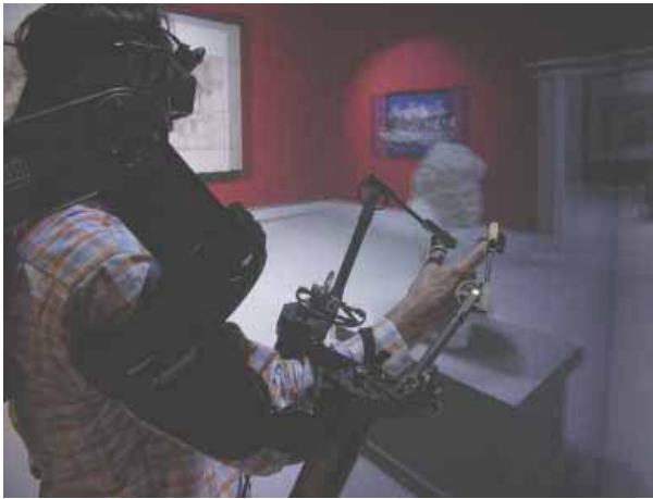
Fig. 4.9. The arm exoskeleton integrated in the C2 configuration
