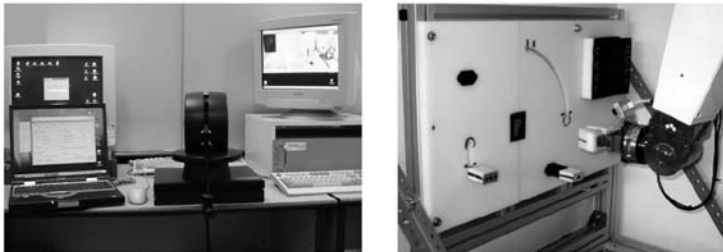
Fig. 17.3. Left: Local Zone, comprised of the master device and the display with the images from cameras. Right: Remote Zone, comprised of robot slave and the task board.
