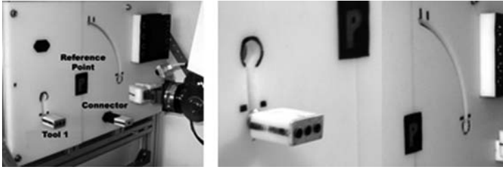
Fig. 17.4. Left: Task Layout, the three phases of the task can be observed: groove movement, insertion and membrane-puncturing. Center/right: Linear/circular groove detail.
