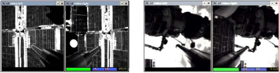
Fig. 19.9. Stereo video images taken by the integrated cameras of ROKVISS showing the robot arm pointing at the solar panel (left) and the Soyuz (right), docked to the ISS
