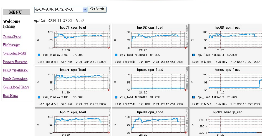
Fig. 3A. Performance data of each computing node involved in computation of PCGrid grid platform
