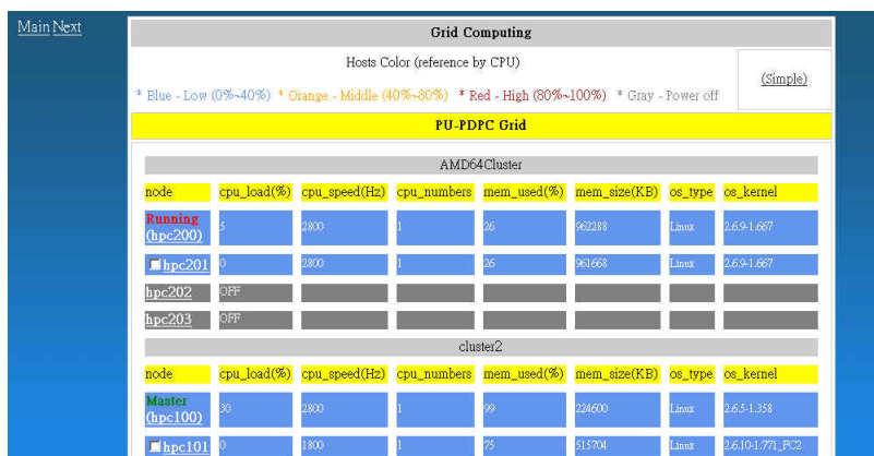
Fig. 2B. Real-time display of all computing nodes status in complete mode
