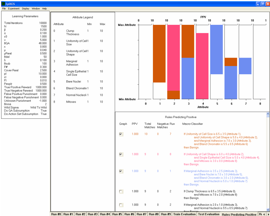
Fig. 6. Rule visualization tool in EpiXCS. Rules are presented in natural language in the bottom pane. Clicking on the checkbox next to a rule causes the values to be plotted in the graphic in the upper pane. Multiple rules can be plotted for comparison and for visual identification of patterns that tend to recur from rule to rule.
