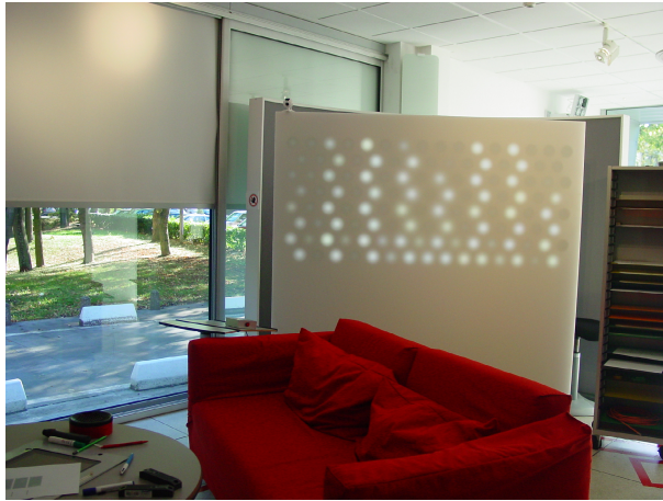
Fig. 4. The Hello.Wall – an ambient display communicating awareness information between different locations via a range of dynamic light patterns
