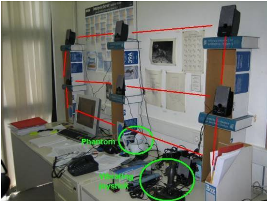
Fig. 2. The current auditory grid (3x3), as it has been prototypically set-up for the King Pong media-space game; a flexible special-purpose construction is underway to encompass the loudspeaker grid (supporting 6x4)
