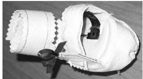
Fig. 2. The BBA bootee with the pulse oximetry system fixed within it.
