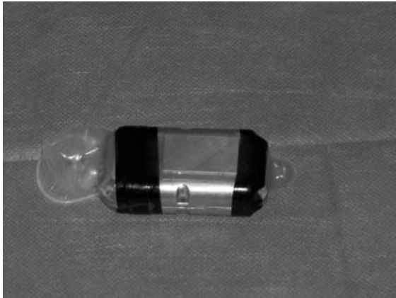
Fig. 3 Implant Case With Patch Antenna Enclosed in Latex Bag
