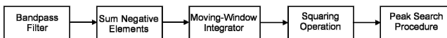
Fig. 8 Block diagram of the peak detection algorithm on the combined dual-axial signal
