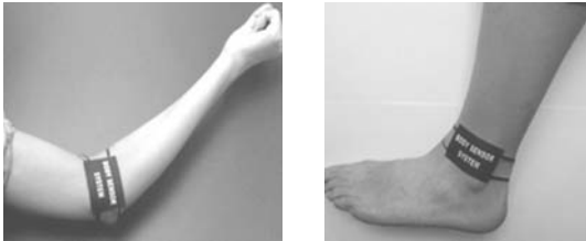
Fig 1 Examples of body movement detection; wireless sensor packs are provided at limb joints to monitor several motion parameters continuously.
