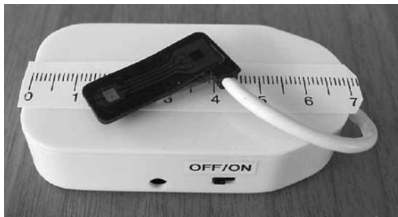
Fig. 1. A sealed, splash-proof box contains all electronic components for measurements and radio transmissions, integrated in the sole of the bootee.
