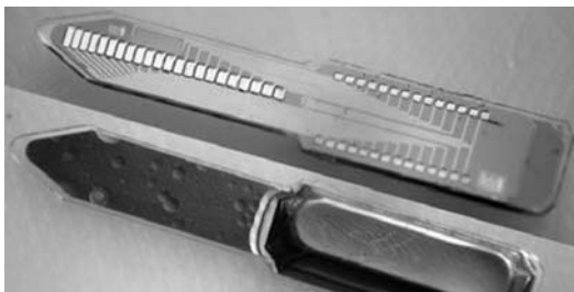
Fig 2 Modiolus electrodes for the cochlear implant
