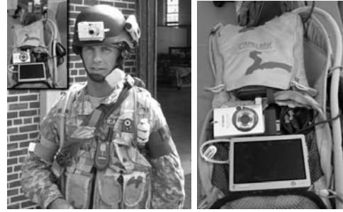
Fig. 2. Left: Soldier wearing the SAS sensor rig at the Aberdeen Proving Grounds. Right: Open Camelbak showing OQO computer and connectors.
