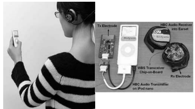
Fig. 12 MP3 File Transfer using On-Body Communication
