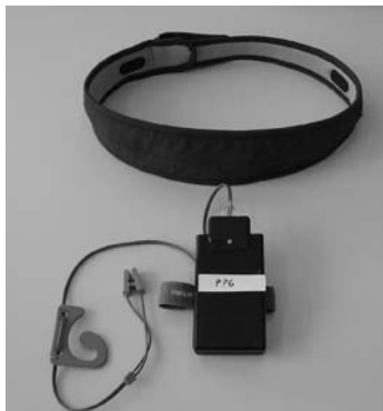
Fig. 2 Wireless ECG belt (top) and PPG ear sensor (bottom)
