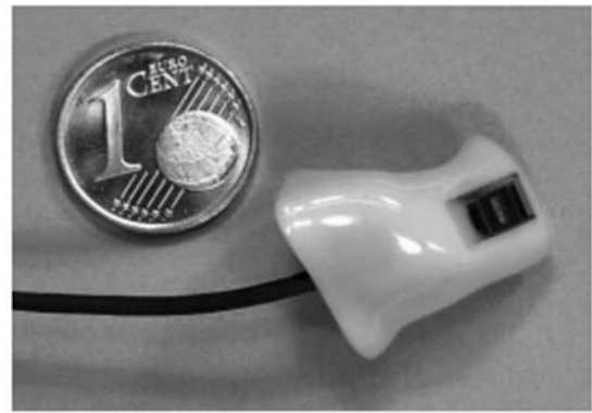
Fig. 8 In-Ear sensor prototype
