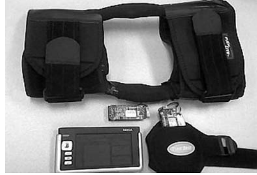
Figure 6: The prototype hardware system includes one base station and two sensor nodes. A knee brace is used for emulating limping context.
