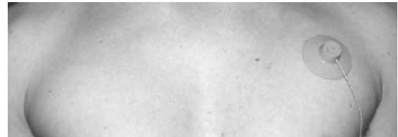
Fig. 4 Microphone capsule on male test person
