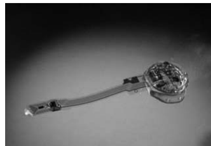
Fig 8 Prototype retina implant
