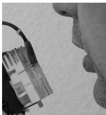
Fig. 7 Experimental set-up for lactate measurement
