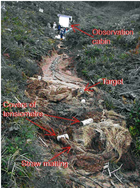
Fig. 15.17. The landslide deposit one day after the experiment
