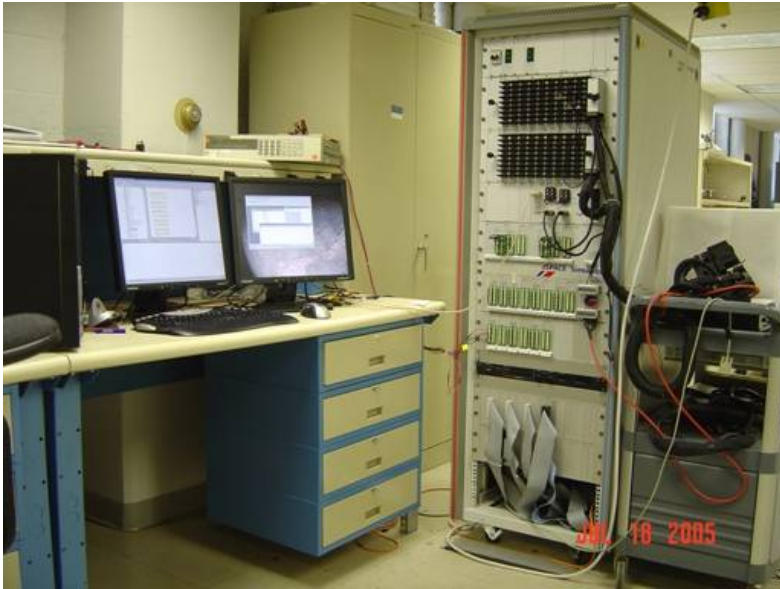
Fig. 2. body electronics hardware in the loop facility
