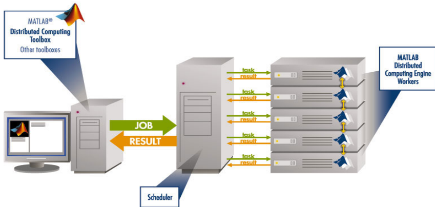
Fig. 6. Developing distributed and parallel applications with the Distributed Computing Toolbox of Matlab
