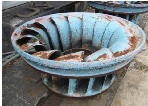
Fig. 2. Cavitation erosion on the old runner.
