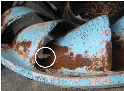
Fig. 7. Cavitation erosion at the blade's leading edge.
