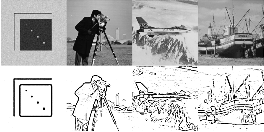
Fig. 3. Four test images and the result of a thresholding process is shown. Since eq.(7) produces both higher ridges and a lower noise level than eq.(8), then the map obtained by the filtering process (8) can be used as a threshold map of the ridge map obtained by the filtering process (7).
