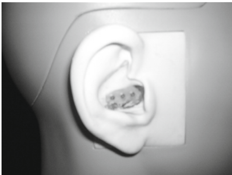
Fig. 16.2. A close up of KEMAR's right ear. The three microphones are placed in the ear and arranged in a horizontal fashion (photo by Ranil Sonnadara).
