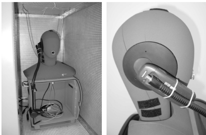
(a) HATS in anechoic chamber. (b) Mobile phone attached to HATS in side view.
