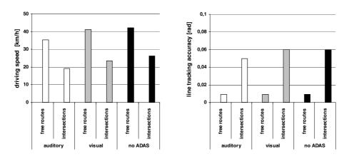
Fig. 3. Effects of ADAS modality on driving speed (left) and accuracy (right)
