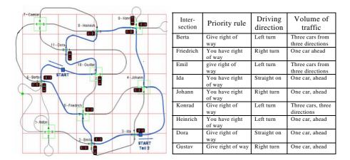
Fig. 2. Left side: Experimental route with nine different intersections; Right side: Priority rule, driving directions and volume of traffic at the different intersections
