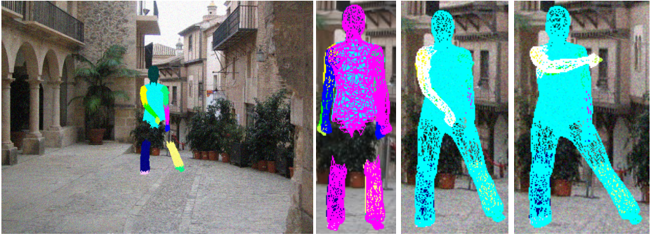
Fig. 3. Simulation of a human that moves an arm in front of its body. Here, every part of the object model was assigned a unique color and projected onto an image of a street in Palma de Mallorca. The only exception are the upper legs, which are transparent to simulate parts on the object that cannot be distinguished from the background. From left to right: (a) Frame 20 of the input sequence. (b) Splitting used in the initial pose in the first frame (magnified). The two components are shown in blue and magenta, respectively. (c), (d) Pose estimation results for frame 20 and 30 (magnified).
