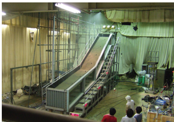
Fig. 20.9 Indoor experiment system of an artificial slope under precipitation control
