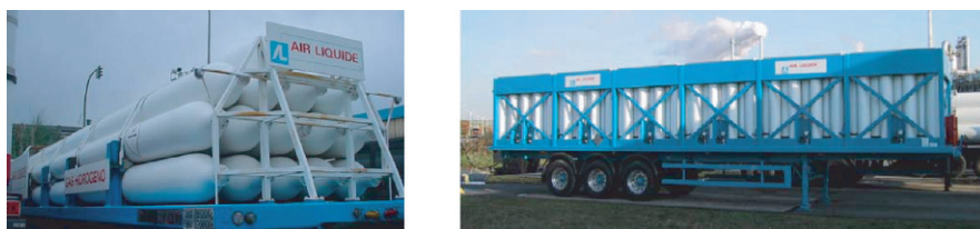
Fig. 4.2 Two types of compressed gas hydrogen trailers operated by Air Liquide in Europe: tube trailer carrying 2000 to 3000 Nm 3 of H 2 (depending on the numbers of tubes) and type II composite cylinder trailers carrying 6200 Nm 3 of H 2 (540 kg)
