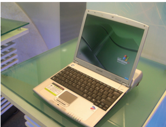
Fig. 13.1 Notebook PC with a fuel cell docking station attached for power supply
