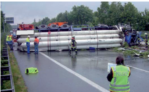
Fig. 9.3 Accident with a compressed-hydrogen-gas tanker in Germany, 2005. The hydrogen bottles remained intact and the hydrogen could be vented safely
