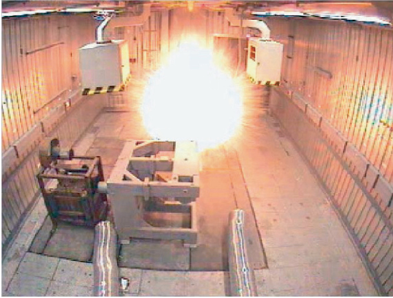
Fig. 9.16 Local explosion of 8 g of hydrogen in the FZK test chamber, simulating an accident scenario in a residential garage
