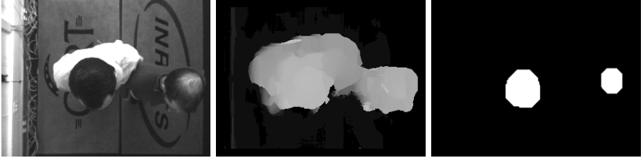
Fig. 2. Example of a height map segmentation (from left to right: initial left image, the height map, the kernels map)
