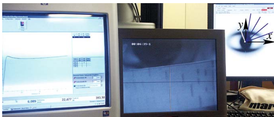
Figure 10.1. USAXS observation during straining of an SBS block copolymer. Right monitor: Intensity maxima on an ellipse. Raw-data coordinate system (x,y) and radial cuts for data analysis are indicated. Middle: Videotaping of sample. Left: Stress-strain curve. Control booth of beamline BW4, HASYLAB, Hamburg
