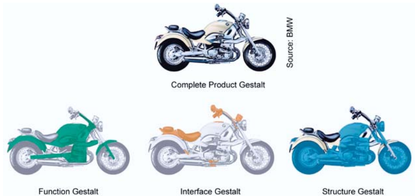
Fig. 3: Function-oriented product structure of a motorbike (gestalts grey shaded)
