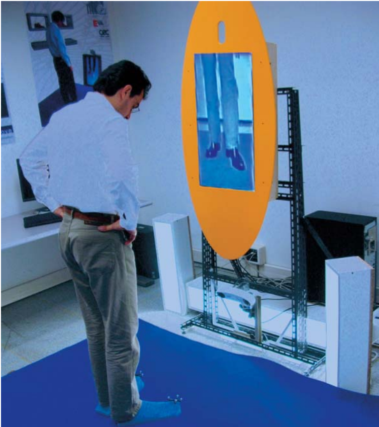
Fig. 2: A blue carpet is replaced by a virtual floor to avoid artifacts
