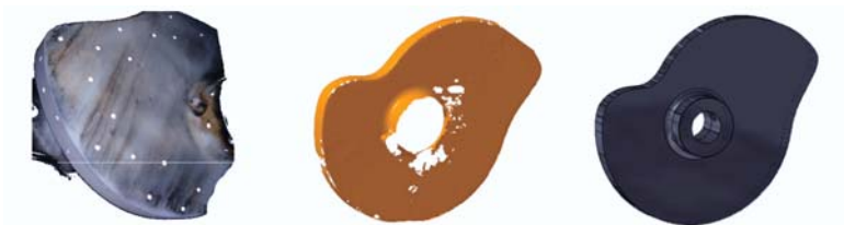
Fig. 3: From physical object to CAD model via cloud of points
