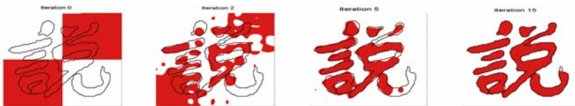
Fig. 3 Evolution of the moving domain \Omega(t) using a Galerkin-Level Set strategy.
