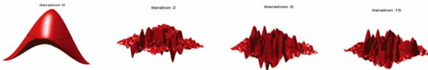
Fig. 4 Evolution of the Level Set function \Phi(t, \cdot) using a Galerkin-Level Set strategy.
