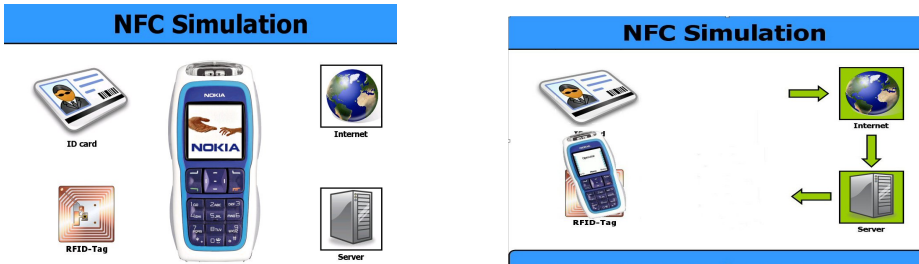
Fig. 8. A created system concept for City of Oulu case in its start and end position. RFID-Tag is touched with the phone and information is retrieved from the Internet.
