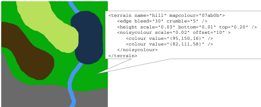
Fig. 3. Landscapes are generated from a terrain map, a simple bitmap image showing where each type of terrain is located
