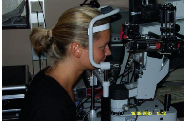
Fig. 9.10 Photograph of the laser interferometer used for the measurement of ocular fundus pulsation
