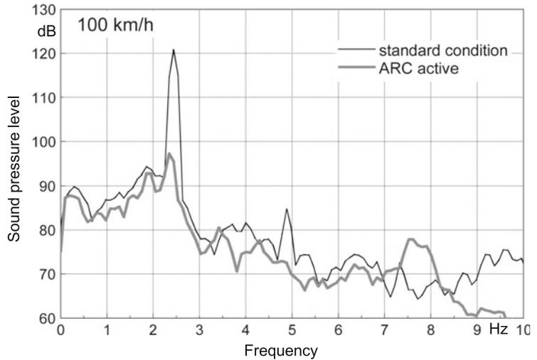
when the active system is applied (Active Resonance Control, ARC, [119].
