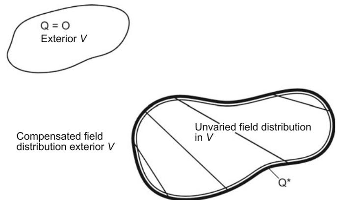
**Fig. 12.10** Compensation of the field in  $V$  without feedback to the outer volume outside  $V$
