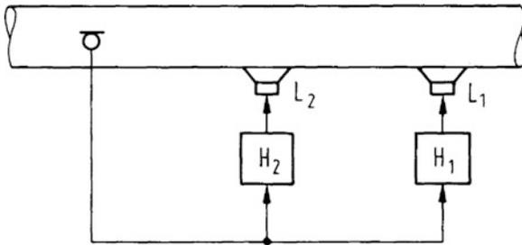
**Fig. 12.14** Active sound field control in channels
