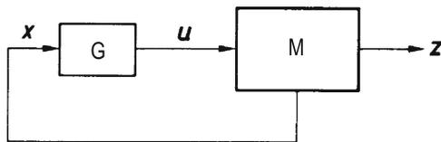
**Fig. 12.31** Principal sketch of the total system and its respective separation into an electromechanical system  $M$  and a signal processing unit  $G$
