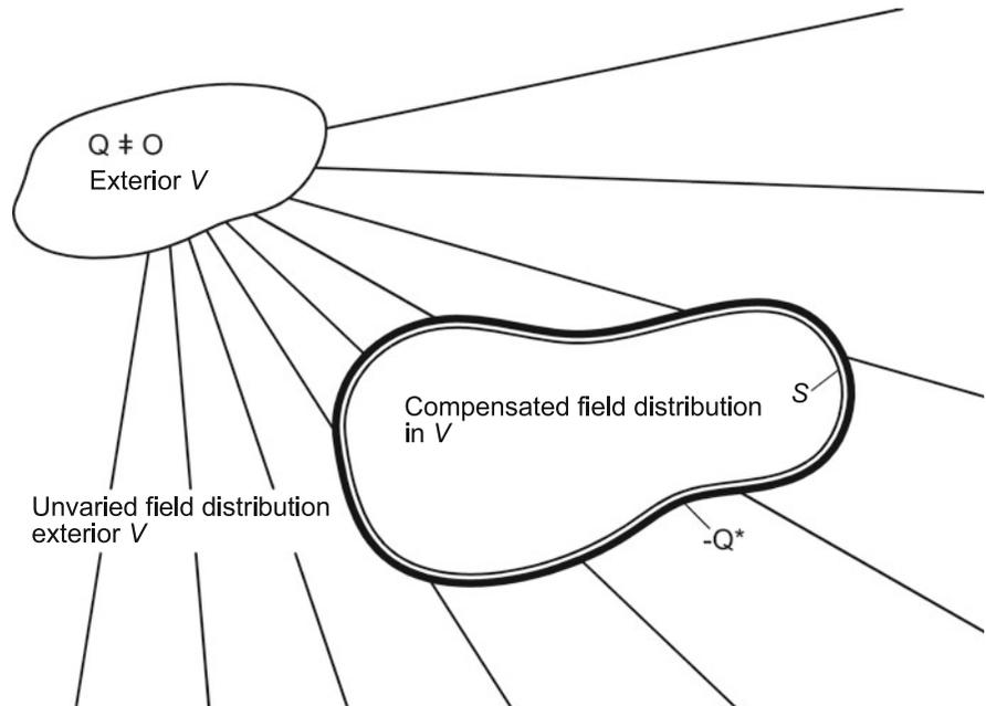
**Fig. 12.11** Purely absorbing field compensation in  $V$
