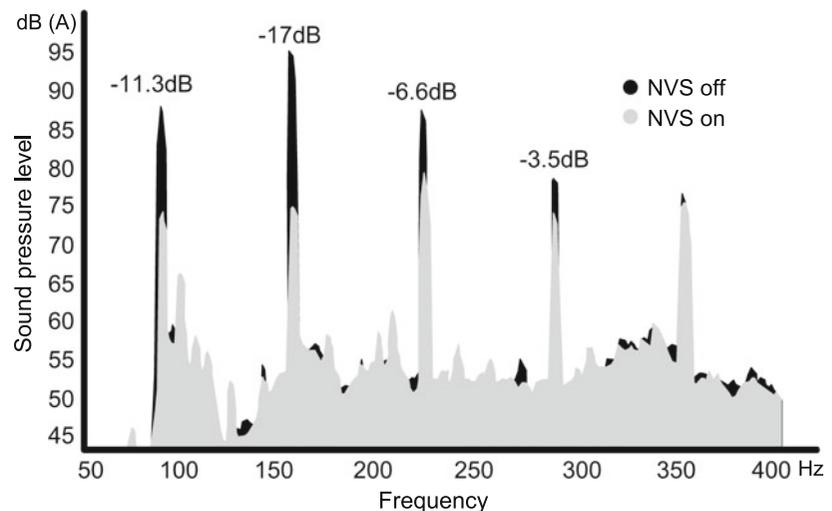
**Fig. 12.24** Sound spectra in a turbo-prop driven aircraft without (NVS out) and with (NVS in) active suppression of sound radiation [109]
