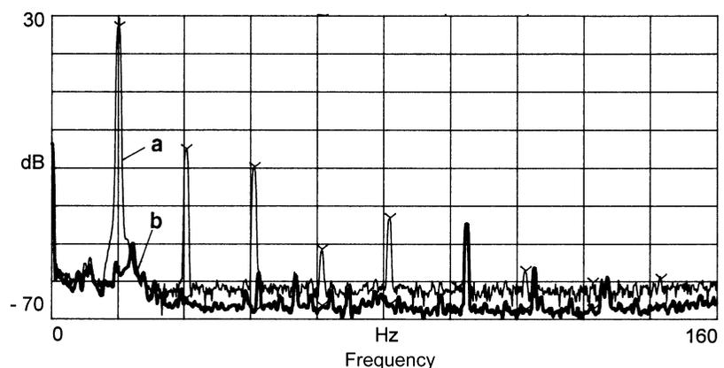
**Fig. 12.33** Frequency spectrum of the force introduced into the foundation (a) without and (b) with active isolation
