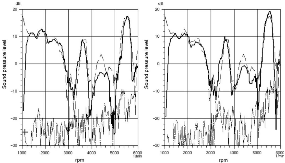
**Fig. 12.29** rpm dependence of the sound pressure related to the third engine order at the driver's (left) and co-driver's (right) seat without (*lower dash-dotted line*) and with (*upper continuous line*) active sound design (ASD). The dashed upper line describes the target to be met by ASD
