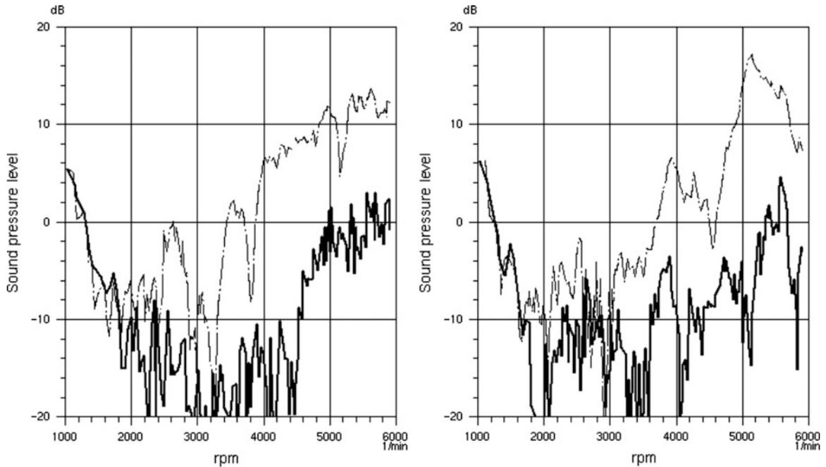
**Fig. 12.21** rpm dependence of the sound pressure caused by the second engine order at the driver's (*left*) and co-driver's (*right*) seat without (*upper curve*) and with (*lower curve*) active noise cancellation (ANC)
