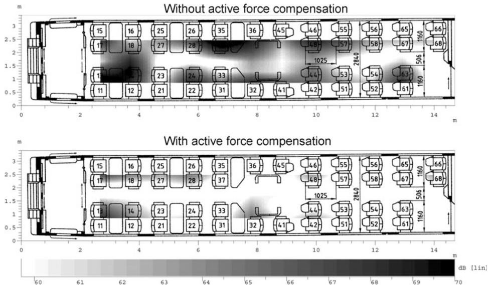
**Fig. 12.6** Spatial sound pressure distribution in the passenger compartment of an ICE passenger train car without (*upper*) and with (*lower*) active force compensation at the bogie's secondary springs
