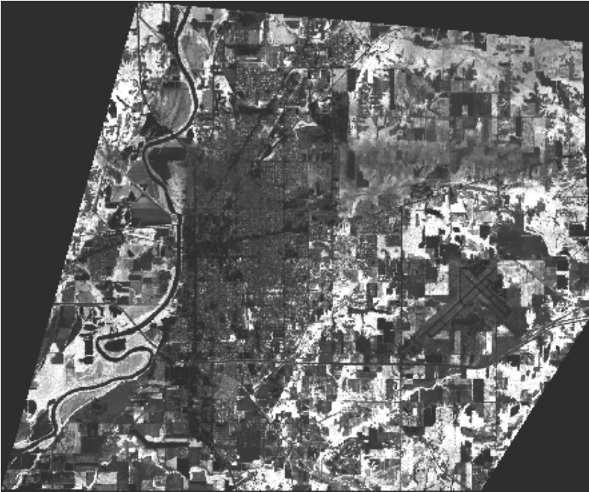
Fig. 2. Estimated LAI map of the Terre Haute area computed using the artificial neural network and three ASTER bands. Lighter areas represent higher LAI values. Note the city center in the middle left of the image and Terre Haute International Airport in the middle right of the image.
