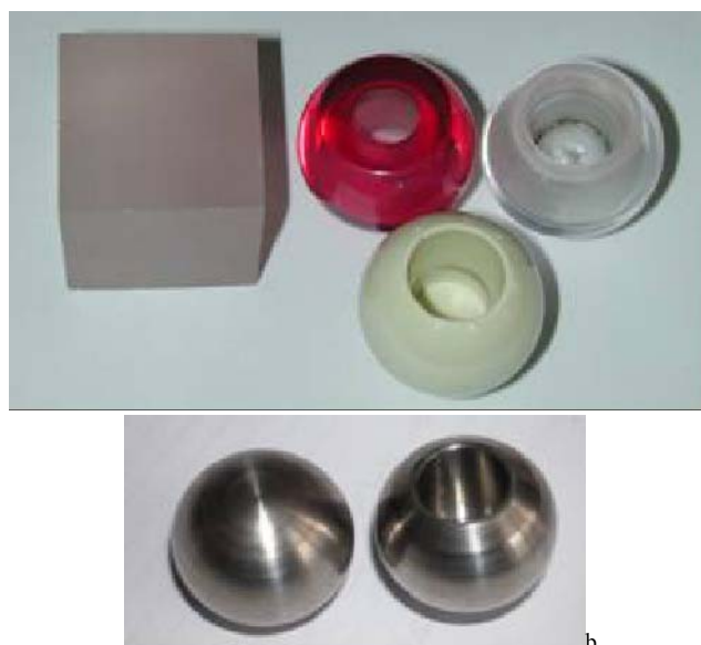
Fig. 1 A blank of sapphire, hip joint heads from sapphire, zirconium ceramics (a) and titanium alloy without V and Al (b).
