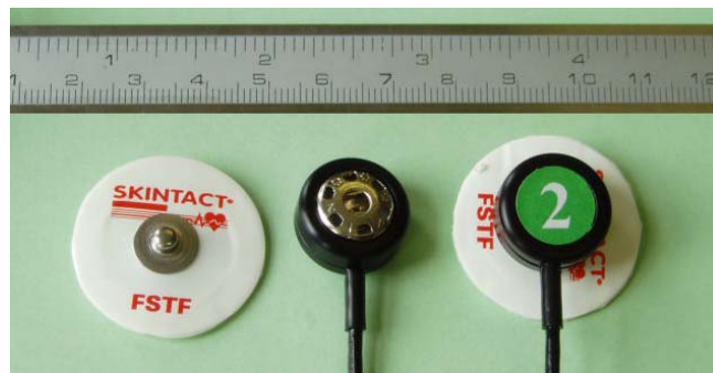
Fig. 1 Active electrodes are composed of quality Ag-AgCl disposable electrodes and active electrode adapter.
