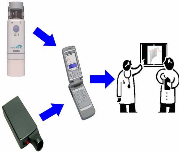
Fig. 2 Telemetric Personal Health Monitoring System for monitoring of bodily functions [4]. In this case the system combines a newly developed aeropneumograph for measuring pulmonary functions with an inhaler for applying medicaments with integrated documentation of the applying times
