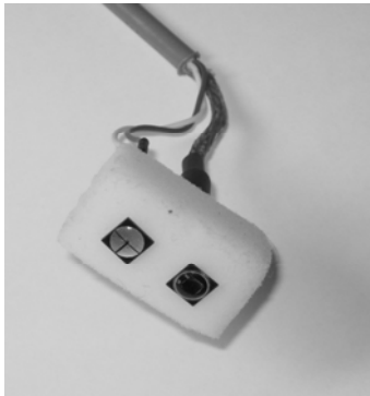
Fig. 3. Reflectance probe for PPG signal measurements.
