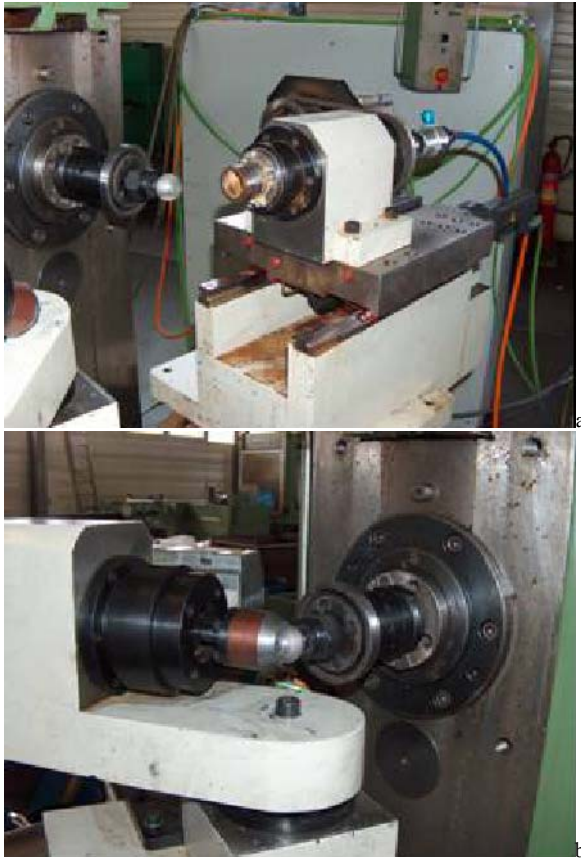
Fig. 2 Preliminary shaping by grinding (a) and finish lapping sapphire hip joint head (b).
