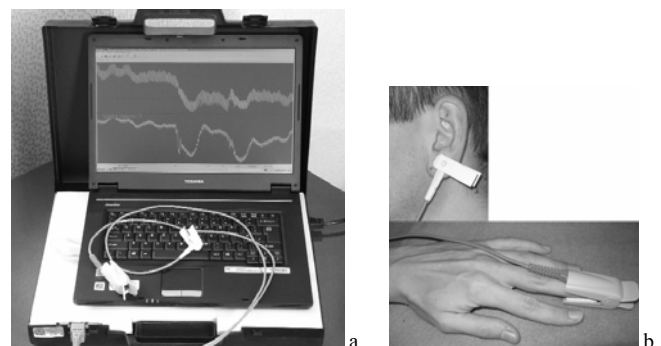
Fig. 1 The PPG device (a) and sensors applied to finger and ear (b).
