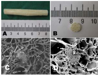
Fig. 2. Observation of the gelatin/silk fibroin hybrid scaffold. (A) gross observation of scaffold; (B) cross section of scaffold; (C) porous structure observed by SEM (×100); (D) Magnified view of the white rectangle frame from (C), demonstrating the hybrid G/SF microsponge around the silk cables (SEM ×150), note: the arrows point to the silk cable and micropores.
