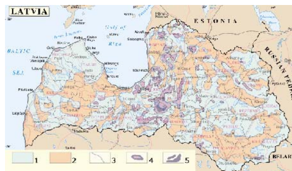
Figure 1.1. Scheme of the anomalous MF in Latvia 1 – positive MF; 2 – negative MF; 3 – zero line of MF; 4 – positive MF with the intensity > 700 nT; 5 – local anomalies containing ferromagnetic minerals.
