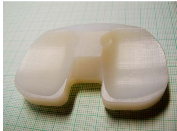
Fig. 1 The polyethylene insert of knee implant.
