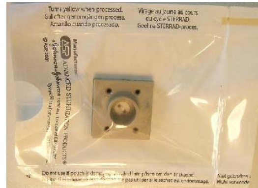
Fig. 1 Sterile packaged BioChip-C with microsensors for measurement of dissolved oxygen, pH, impedance and temperature. The side length of the chip is 24 mm.
