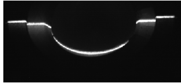
Fig. 4 Recorded digital image of the linear strip deformed by the surface.
