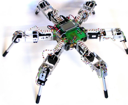
Fig. 3. Experimental hexapod robot OSCAR (Organic Self Reconfiguring and Adapting Robot) has six legs, with three motors per leg. Going from the body – alpha, beta and gamma.
