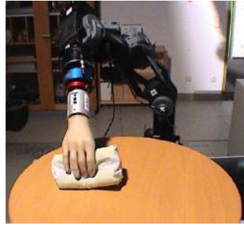
Fig. 9.1. DLR-Lightweight-Robot-II in a table wiping application
