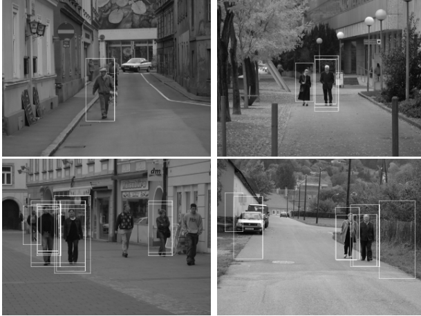
Fig. 5. Examples of pedestrian detection. In upper image pedestrians are correctly detected. Lower images show example of false detection.
