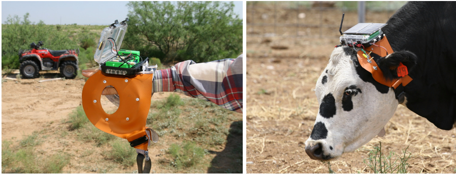
Fig. 1. The sensing and actuation box [8] is roughly 21.5\text{cm} \times 12.0\text{cm} \times 5.5\text{cm} and weighs around 1kg. It is equipped with a GPS receiver, wireless networking features, and a suite of sensing and actuation capabilities. The Lithium-Ion batteries and solar panel allow for indefinite operation under normal conditions. The sensor box is mounted to the head of a cow with a leather strap designed to use the cow's ears to keep the box in position. Pictures courtesy of I. Vasilescu.
