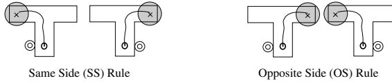
Fig. 1. A schematic representation of the delayed response rules. Light samples are represented by double circles. Target locations are represented by \times , while reward corresponds to the gray area. The behavioral task asks for controllers capable of switching between the two rules.
