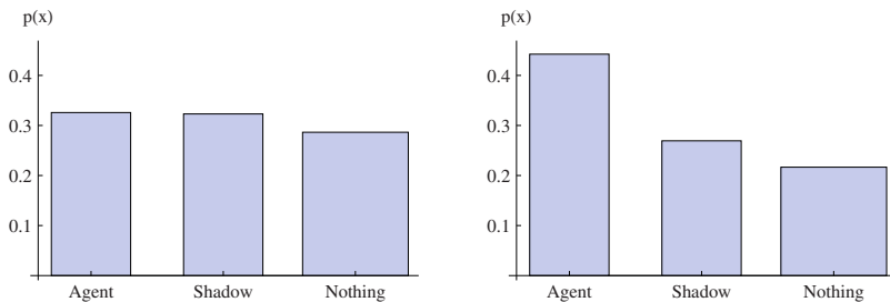
Fig. 3. Normalized interaction time of agent A with agent B, with the shadow of agent B, and with neither of the two, respectively for runs of 60 minutes simulated real time. (left) Self-organizing behavior according to the homeokinetic principle without rewards. (right) Homeokinetic learning with additional reinforcement of situations where tactile input was received.
