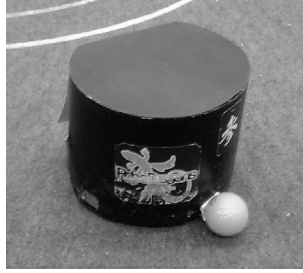
Fig. 10. A robot and a ball that are used for occlusion experiment
