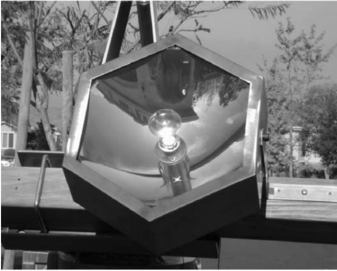
Fig. 6.8. Photograph of a single assembled concentrator unit during testing
