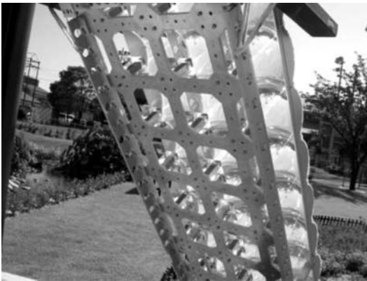
Fig. 15.22. A CPV for ‘breeding plants’ that collects direct beam and provides diffused sunlight to the plant underneath
