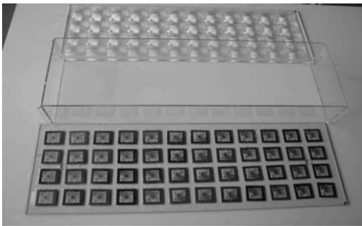
Fig. 14.2. Operating principle of the FLATCON technology. The light is concentrated on a tiny cell. The cell is mounted on a copper heat sink which facilitates passive cooling. It is noteworthy that the copper area is similar to the lens area. This guarantees similar thermal behaviour to a flat-plate module, even though highly concentrated light is used
