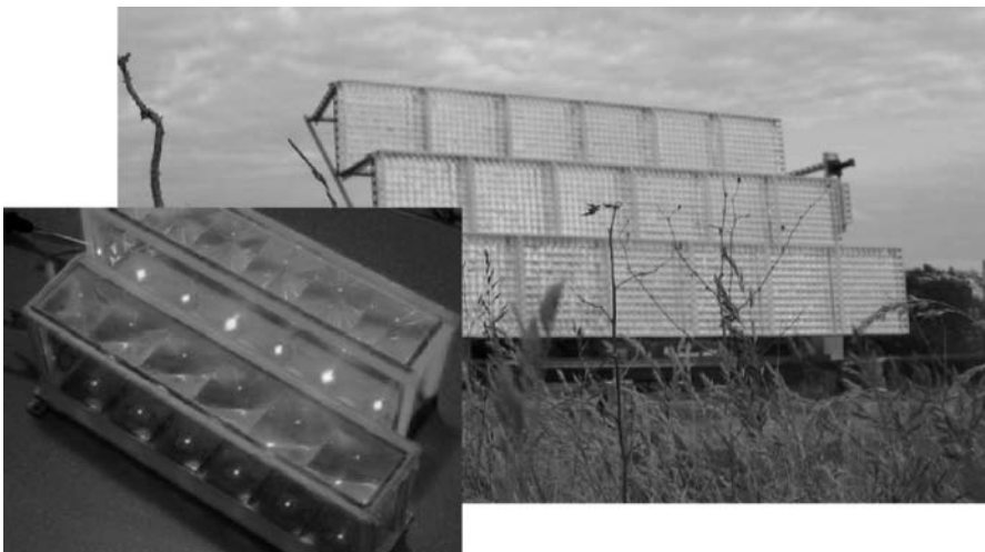
Fig. 8.20. The experimental modules with solar GaInP/GaAs/Ge triple-junction cells and AlGaInP LEDs, both equipped with small-aperture-area Fresnel lenses and being under forward bias conditions [17]; similarity of main features, favourable for promotion of both LED lighting arrays and solar concentrator modules
