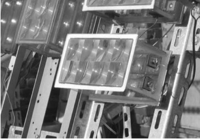
Fig. 8.17. Arrangement of the eight-lens module with Spectrolab's cells on a sun tracking system
