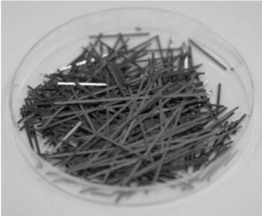
Fig. 3.6. Slivers, each 1 mm wide and 50 \mu\text{m} thick
