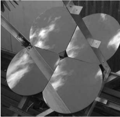
Fig. 9.2. Pseudo-parabolic facet concentrator made of four spherical dish mirrors installed on a sun tracker
