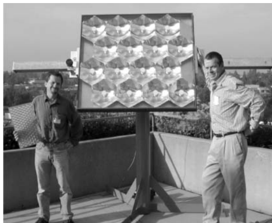
Fig. 6.1. Prototype modules of two generations of commercial high-flux PV concentrators. Right: module comprising 16 identical dual-mirror concentrators each 310 mm across and transmitting 50 W onto a 100 mm 2 triple-junction solar cell [9]. Left: all-glass counterpart, constituting 160 identical concentrators, each 31 mm across, with 0.5 W irradiating a 1.0 mm 2 ultra-efficient triple-junction PV. Both modules are essentially achromatic, with an aspect ratio of about 1 to 4. (Courtesy of the SolFocus Corporation, Palo Alto, Calif.)
