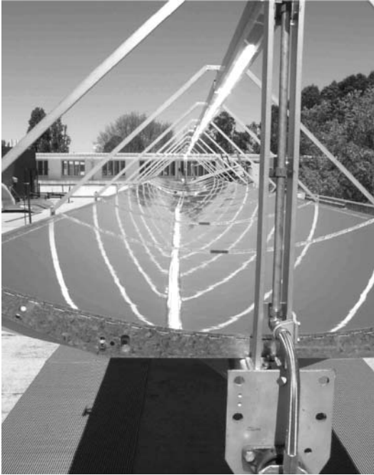
Fig. 3.5. Parabolic trough concentrator, illustrating the shadows cast on receivers by gaps between the mirrors and structural elements
