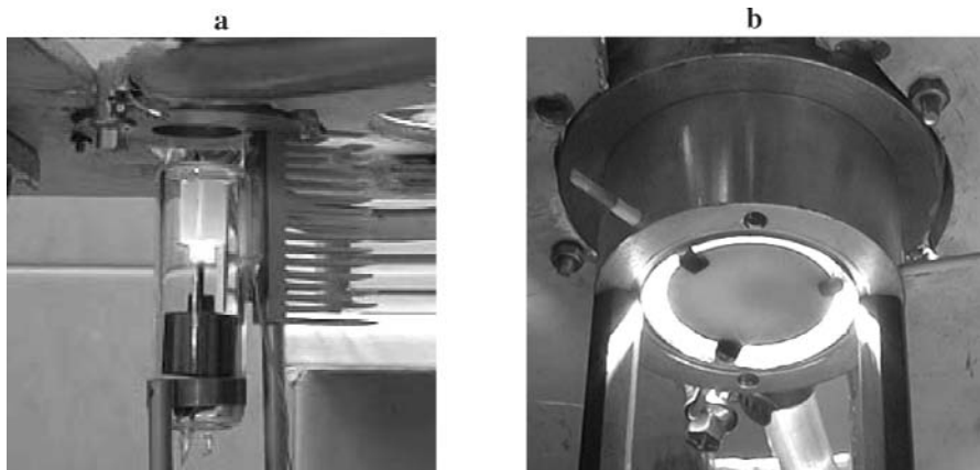
Fig. 9.20. a Part of a cylindrical TPV module with a tantalum emitter situated in an Ar-filled bulb under illumination from solar simulator. b Conical module with a SiC flat emitter installed and heated with the solar simulator
