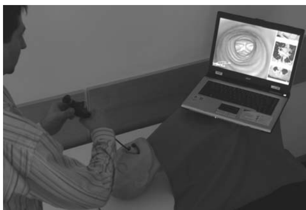
Fig. 3. The user holds a real endoscope in his hand in order to „fly“ virtually through the original CT data. The position and orientation of the endoscope are tracked via potentiometer and used to render a 3D image during movement, thus generating a realistic impression. The prototype is ideal for learning purposes in order to find possible pathologies employing individual patient data. Exercising of taking a biopsy at critical locations or reaching tumors difficult to access can also be practiced by the specialist before operation.
