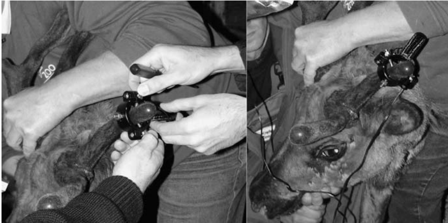
Fig. 7. Fixation of the device to the antler of a reindeer in Duisburg zoo. The animal stayed calm without any anaesthesia.
