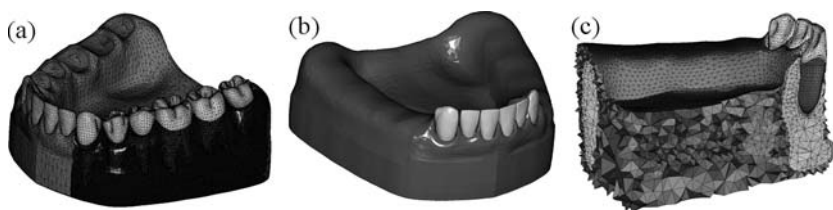
Fig. 1. (a) Surface model of the lower jaw with incorrect modeled alveolae and fully modeled teeth. (b) Surface model of the jaw after removing all molars and premolars and modeling the effect of an atrophy. (c) Resulting FE model of the left half of the jaw, including bone and periodontal ligament.
