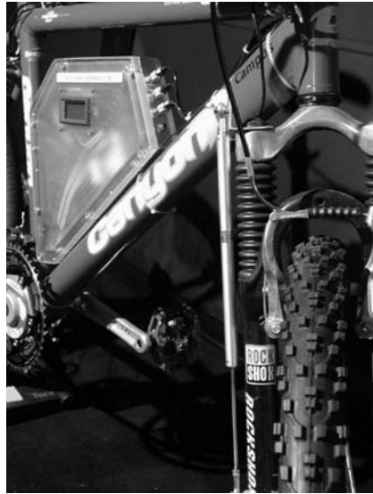
Fig. 2. Data-Recording-System attached to the bike frame.
