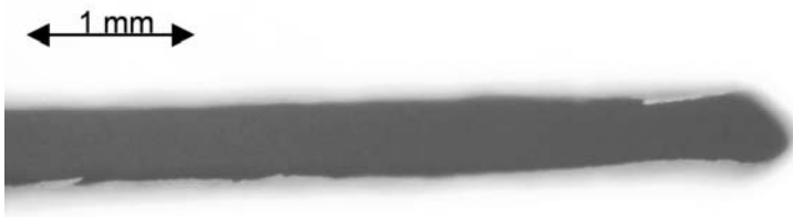
Fig. 6. Bone cut with laser with water spray application and beam scanning
