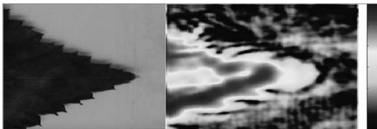
Fig. 6. Leaf in reflection configuration at 260 GHz (Scan area about 25 mm by 25 mm).
