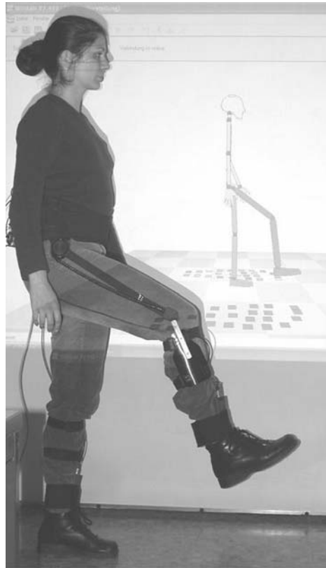
Fig. 2. Online display of the measured data: In the foreground subject with pressure insoles and angle encoders. On the screen behind: Visualization of the measured angle and pressure data using an animated figure and pressure distribution arrays
