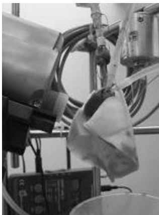
Fig. 4. Isolated perfused and ventilated rabbit lung, on the left side the OCT 3D scanner head can be seen
