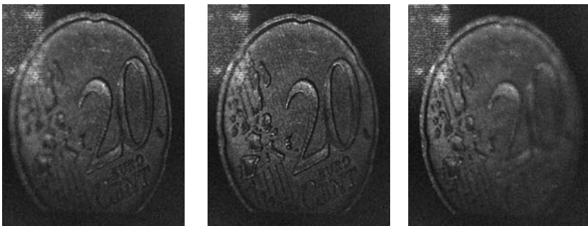
Fig. 3. Reconstruction of a 20 cent coin recorded in a distance of about 40 cm. Reconstructed from left to write in 39,7 cm, 41,1 cm and 43,6 cm distance.
