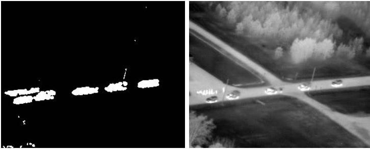
Fig. 2. Background modeling does not work as well for detecting people because the people appear as very small regions that are indistinguishable from clutter noise.
