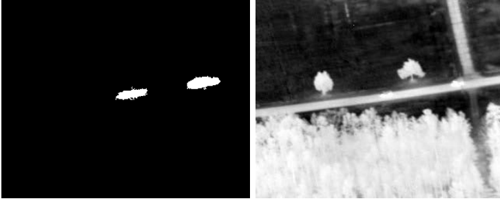
Fig. 1. Background modeling is an effective method of detecting vehicles. Since the vehicles are large and fast-moving, they appear in the subtraction image as large, clearly separated segments.
