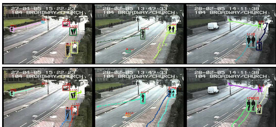
Fig. 13. Sample tracking results obtained with and without blob splitting using projection histograms. Top row: without blob splitting. Bottom row: with blob splitting.
