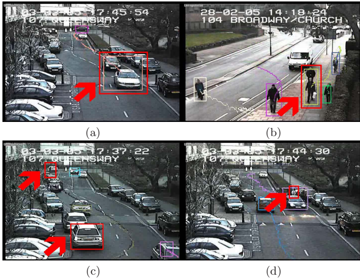
Fig. 15. Sample failure modalities on the CLEAR Broadway Church (BC) and Queensway (QW) scenarios (red boxes indicate the areas of the frame where the failure occurred). Top row: merged objects. Bottom left: missed detections caused by small objects. Bottom-right: object incorporated into the background model.
