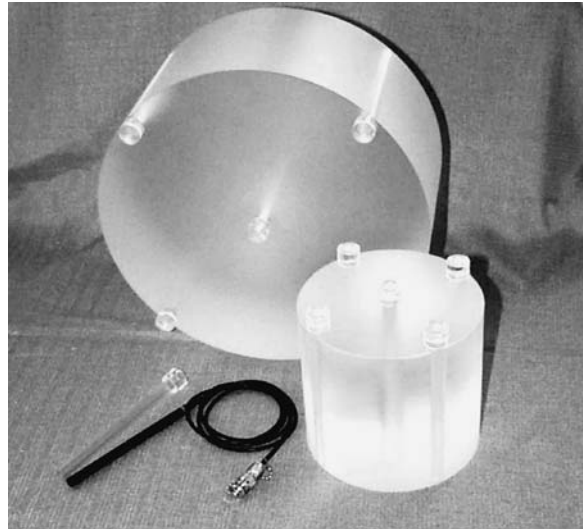
Fig. 4.4. Cylindrical standard computed tomography (CT) dosimetry phantoms (16 cm and 32 cm in diameter) made from Perspex for representative measurements of the computed tomography dose index (CTDI) in regions of the head and the trunk, and a pencil-like detector for measurements of the dose-profile integral
