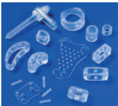
Fig. 17.11. Polylactic acid radiolucent resorbable implant devices: plates; cages; and screws. (From Neurosurgical Focus , American Association of Neurological Surgeons)
