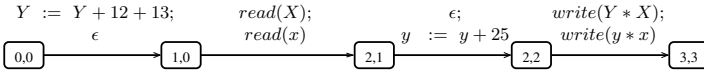
Fig. 1. A comparison transition graph for f(\&(Y, y)) . We use capital variables to denote the variables of the source and their lower case counterparts for the target.
