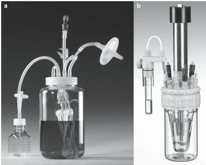
Fig. 5.3 Special bioreactors for small-scale and process development. (a) Superspinner, Membranreactor with tumbling membrane basket for bubble free aeration, Sartorius AG, Prof. Lehmann, University of Bielefeld (courtesy of Sartorius AG, Germany); (b) conical reactor (courtesy of medorex, Germany)
