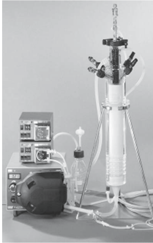
Fig. 5.25 Fluidized bed reactor E500 (courtesy of Cellonic GmbH, Germany). Culture volume: 300–1150 ml; Microcarrier bed volume: 50 mL to 500 mL
