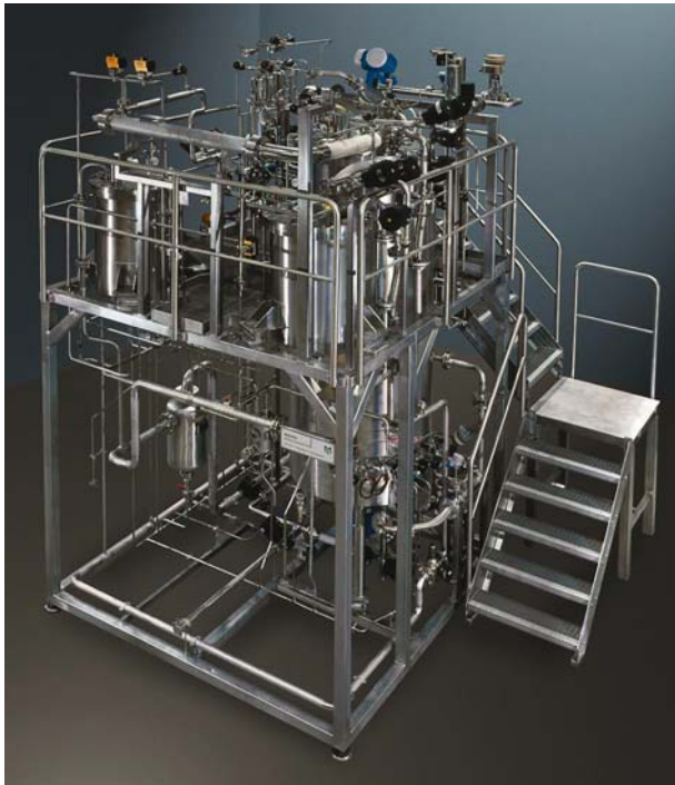
Fig. 5.8 Production-scale bioreactors for cell culture (courtesy of Zeta AG, Switzerland)
