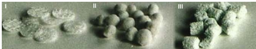
Fig. 4.30 Macroporous carriers for fixed bed and fluidized bed. I: Fibra-Cel™ (New Brunswick); II: glass carrier SIRAN® (QVF); III: ceramic carrier SPONCERAM® (Zellwerk)
