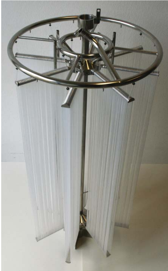
Fig. 4.25 Photograph of the dynamic membrane aeration system (DMA) for a 200 L cell culture reactor (with courtesy from Bayer Technology Services GmbH, Germany)
