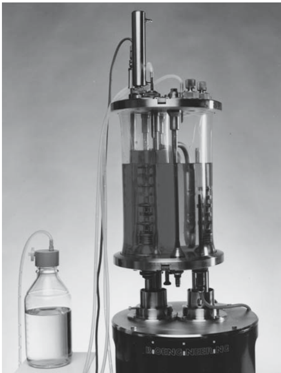
Fig. 5.18 Membrane-dialysis reactor (Prof. Märkl, TU Hamburg-Harburg & Bioengineering AG)
