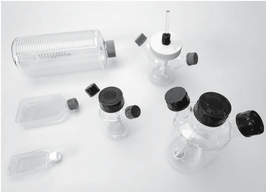
Fig. 5.2 Cultivation systems (flasks, roller bottles and spinner flasks) for use in incubator or warm room
