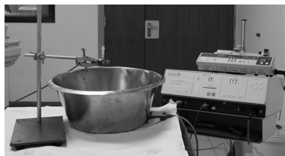
Fig. 3 The experiment setup showing how the biopsy needle is connected to the RF generator using the adapter developed.
