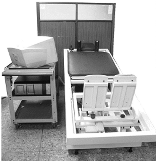
Fig.2 Developed system consisting of a tilt table and patient monitor.
