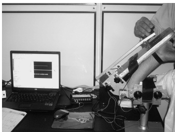
Fig. 1 Passive measurement of stiffness simultaneously with SEMG.
