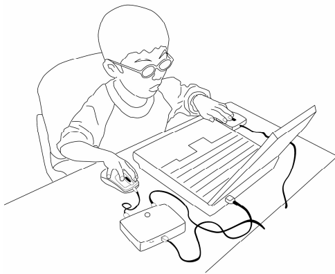
Fig 2. One Child with Cerebral Palsy Operates the Mouse via an Integrated Pointing Device Apparatus. He Used One Mouse for Cursor Control with Dominant Hand and Used an External Switch for Click Control with the other Hand Simultaneously
