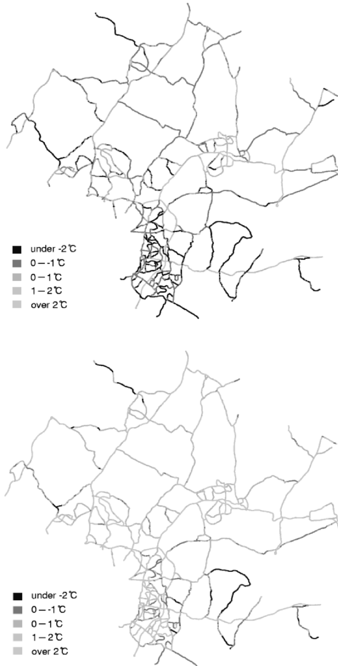
Fig. 22.2. Temperature distributions for two nights in South Gloucestershire: on a cold night (UPPER) and on a marginal night (LOWER)
