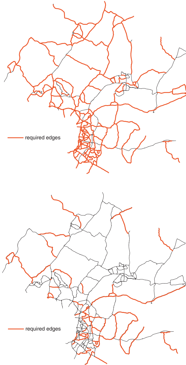
Fig. 22.5. Required edges for Fig. 22.2: on a cold night (UPPER) and on a marginal night (LOWER)
