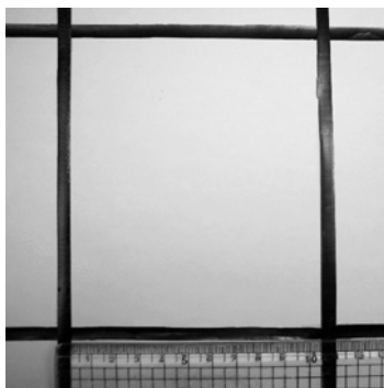
Figure 19.16 Spray-on carbon nanotube neurons in a grid pattern for environmental monitoring
