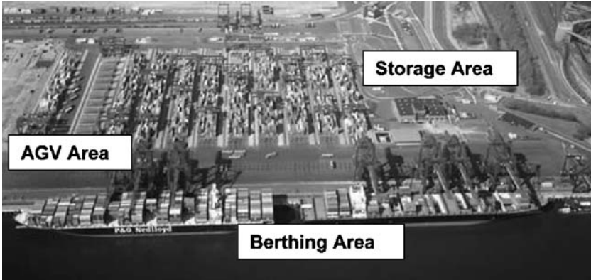
Fig. 2 Layout of the Container Terminal Altenwerder, Hamburg, Germany (source: http://www.hhla.de/de/Geschaeftsfelder/HHLA_Container/Altenwerder_(CTA)/Daten_und_Fakten.jsp , visited on August 22, 2005)
