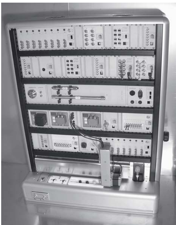
Fig. 10. Modular system components combined in aluminum rack
