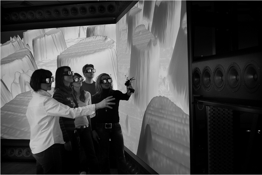
Fig. 16.17. CAVE-like environment with WFS (courtesy of the Fraunhofer Institute of Digital Media Technology (IDMT) and Technical University Ilmenau, Engineering Design Group)
