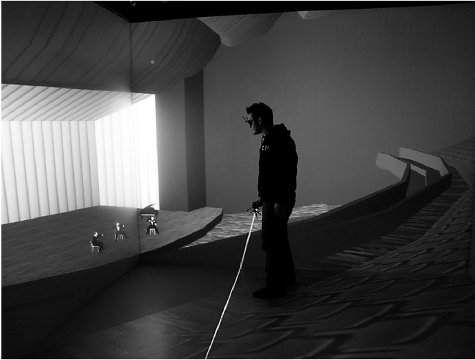
Fig. 16.2. Concert hall model in a CAVE-like environment (CAVE TM Automatic Virtual Environment)
