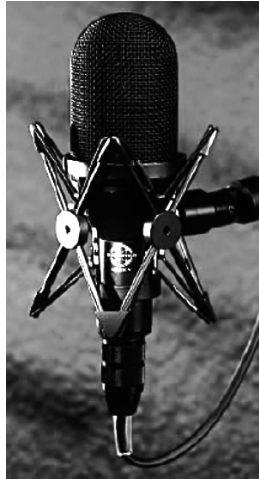
Fig. 16.12. Sound field microphone for recordings in B-format (courtesy of Lab. of Acoustical Imaging and Sound Control, TU Delft)
