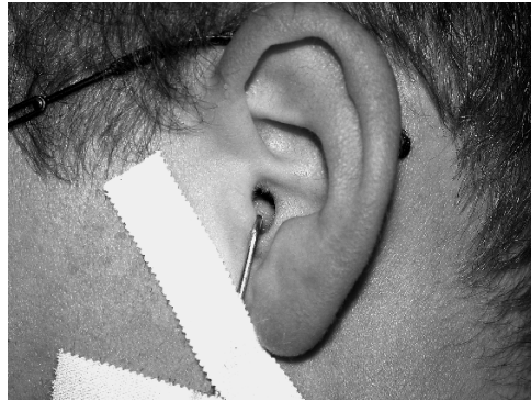
Fig. 16.10. Probe microphone in the ear canal of a test subject
