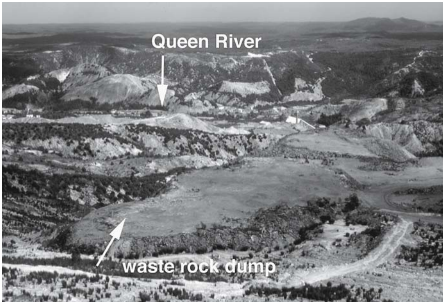
Fig. 3.10. Unvegetated waste rock dump at the Mt. Lyell copper mine, Queenstown, Australia. Waste rock dumps and mine workings are significant sources of AMD into the Queen River. It has been estimated that AMD will continue for another 600 years with the present copper load being 2 000 kg per day (Koehnken 1997)
